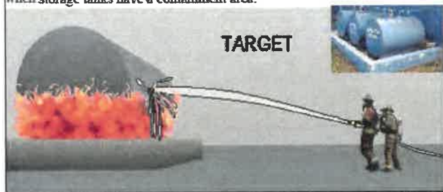
Banking/lobbing may be used to insulate other surfaces.
